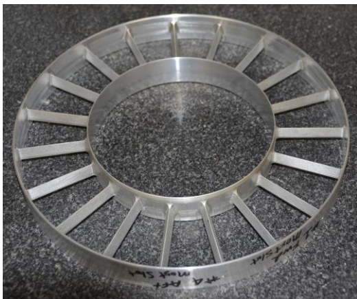
(a) Bars used in the experiments for inlet distortion
